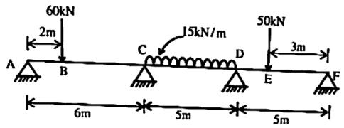
Q.6 Determine the slope and deflection at point B ( $\theta_B$ ,  $\Delta_B$ ) and at point D( $\theta_D$ ,  $\Delta_D$ ) using Conjugate Beam method for the beam given below. Take E = 70GPa and  $I = 700 \times 10^6 \text{mm}^4$
