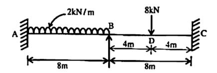
Q.3 Analyze the two span continuous beam by using the Clapeyron's theorem. Draw the shear force and bending moment diagrams.
