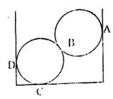
Q.2 Block A weighing 1000 N rests over block B which weighs 2000 N as shown in Figure.
